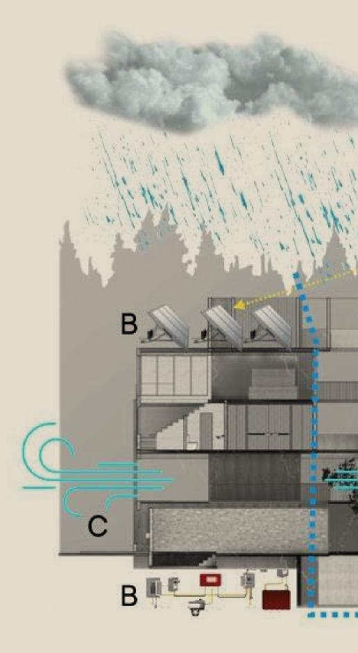
MIRVAL counts with solar panels to convert sun light to electric energy, along with two elecricity generators thet will power the building for up to 14 hours. It will also count with a system to collect rainwater, that will be treated and reused in common areas and outside green areas.
